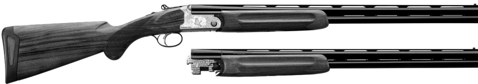
Figure 1.14 The Benelli Renaissance Classic, an over/under configured shotgun. The 20- and 28-gauge barrels are shown. (Image courtesy of Benelli USA.)
